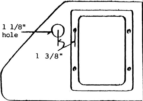
View: R H rear engine baffle, looking forward.
