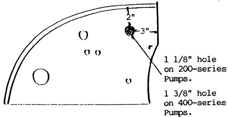
View: L H rear engine baffle, looking forward.
