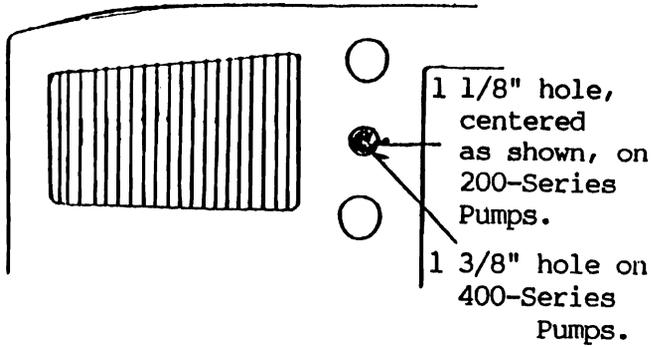
View: L H rear engine baffle,
